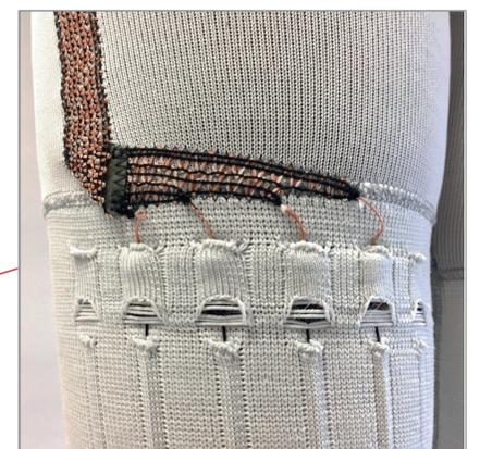
Fig. 4: Bandage with conductor tracks and integrated sensor threads
