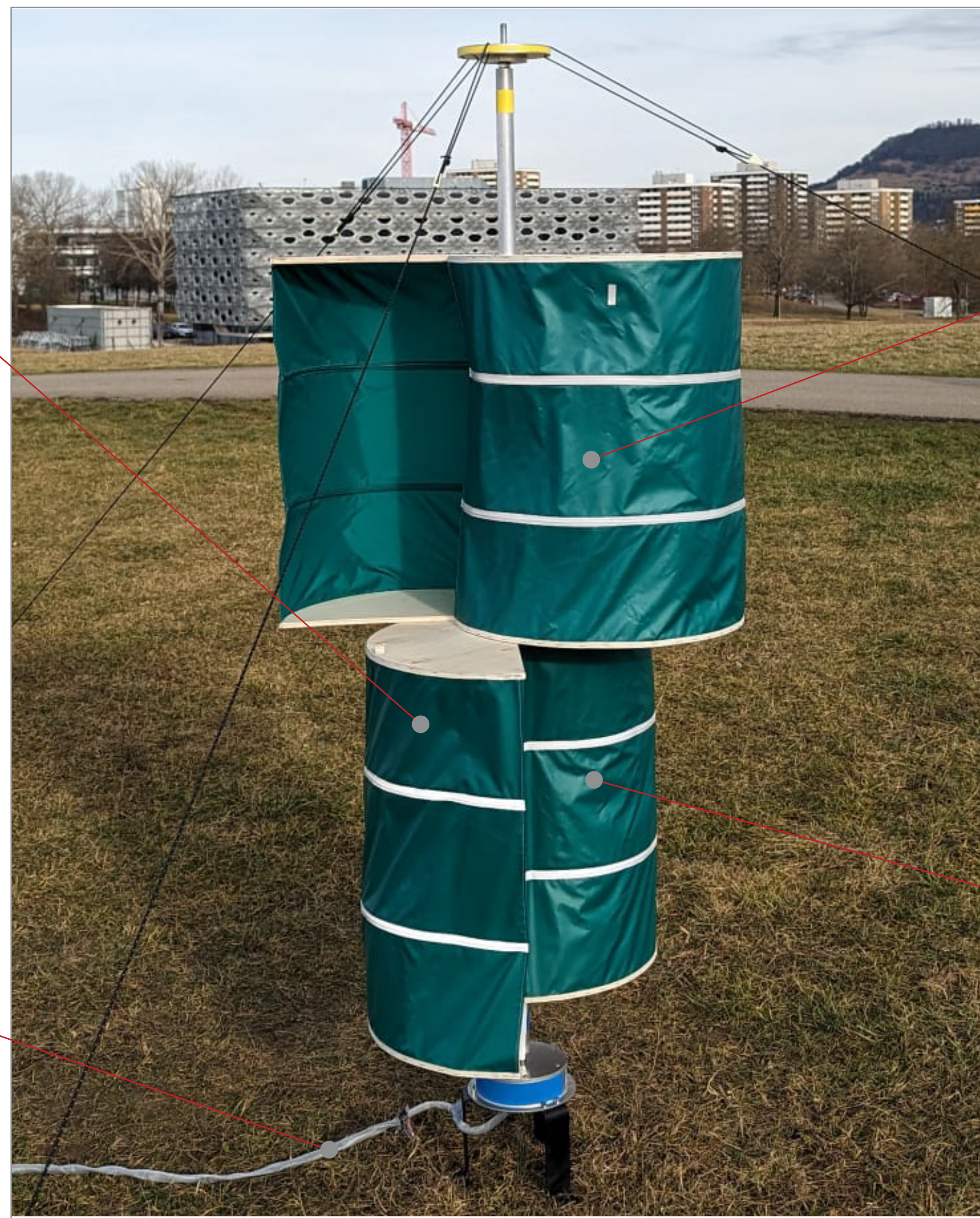
Fig. 6: Functional model of a portable wind turbine with textile components
