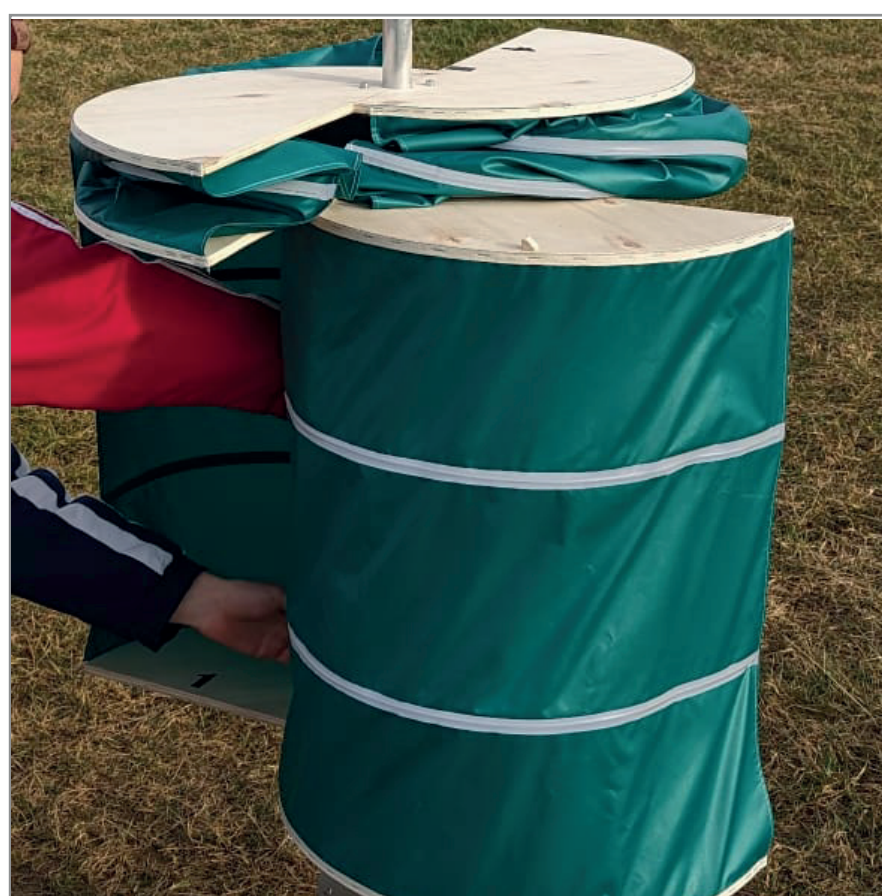
Fig. 2: Deploying process of the rotor during assembly
