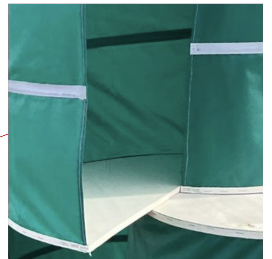
Fig. 4: Textile rotor consisting of windproof fabric and reflective details
